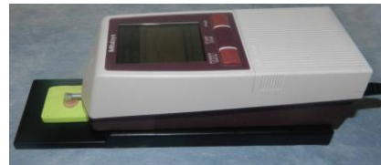
Figure 2. Representation of surface roughness evaluation with the tactile profilometer
