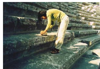
Figure 7. Color measurement at the Aspendos Theater from Cavea (Lower section seating rows)
