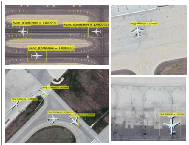
Fig. 8. Aircraft detection results of RCNN testing
