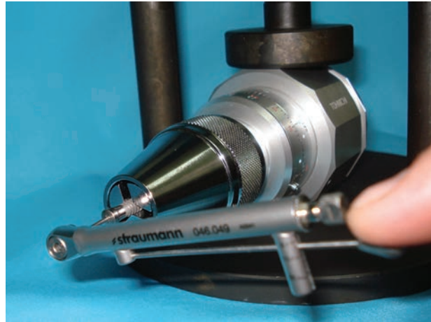
Figure 1. Torque delivery accuracy measured using a technique that simulated the clinical situation
