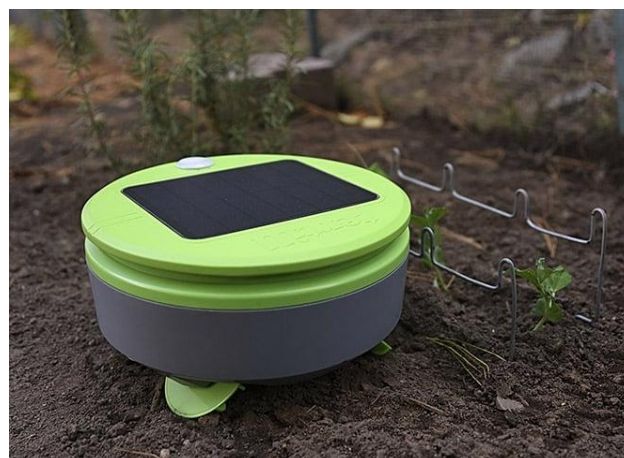
Figure 4- Tertill robot (Sanchez & Gallandt 2021)
