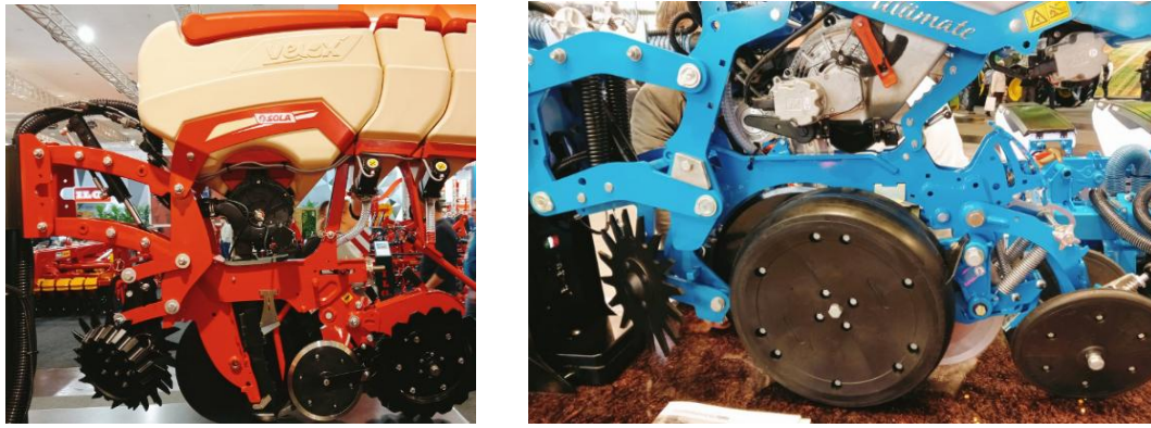
Figure 1. Planter units designed for no-tillage.
