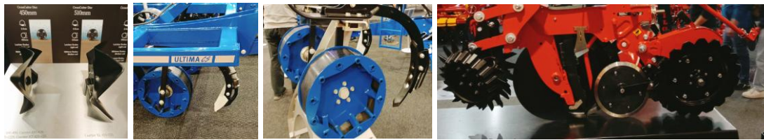
Figure 2. Furrow opener and disc models developed for no-tillage planters.
