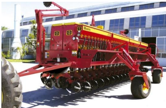
Figure 7. The transport system of the planter developed by Bertini (transport mode).
