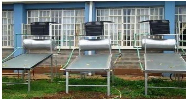
Figure 5. Photo of the experimental setup of solar water heating systems (A, B and control system C)
