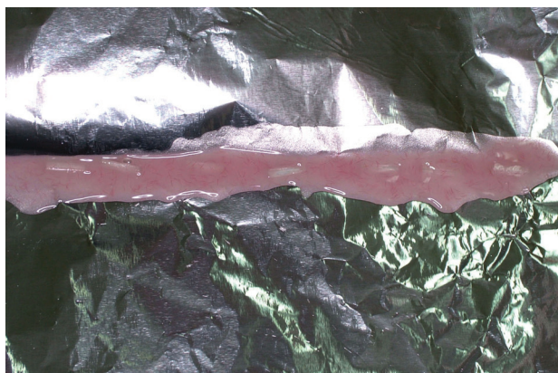
Figure 2B. Impregnation of the e-glass fibers in an aluminum foil
