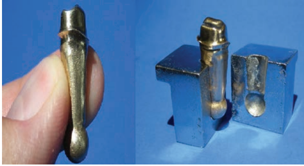
Figure 1. Metal die sample with cross section root design.
