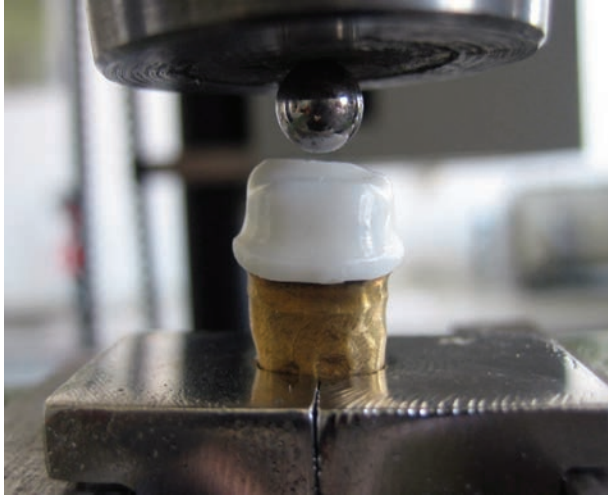
Figure 5. Static fracture strength testing of zirconia core with a universal testing machine.
