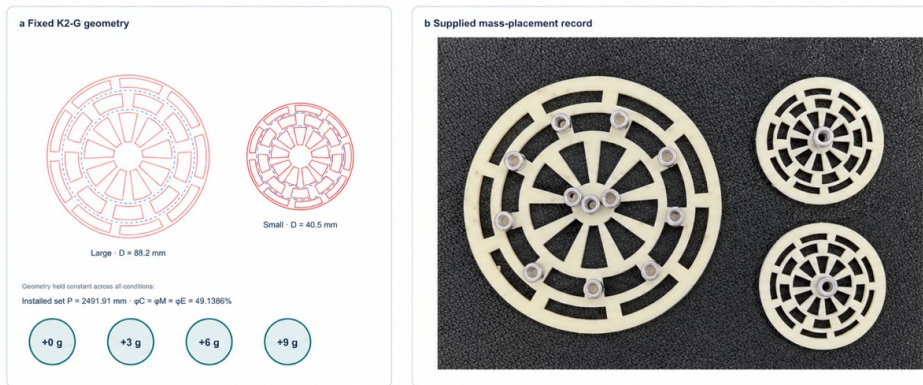
Figure S7. Added-mass experiment based on the fixed K2-G component set for M0, M3, M6, and M9. The source photograph documents mass placement. The measured baseline rosette-set mass was 15.8 g; nominal added masses were 0, +3, +6, and +9 g. The added masses are experimental increments and are not estimates of the total installed assembly mass.
