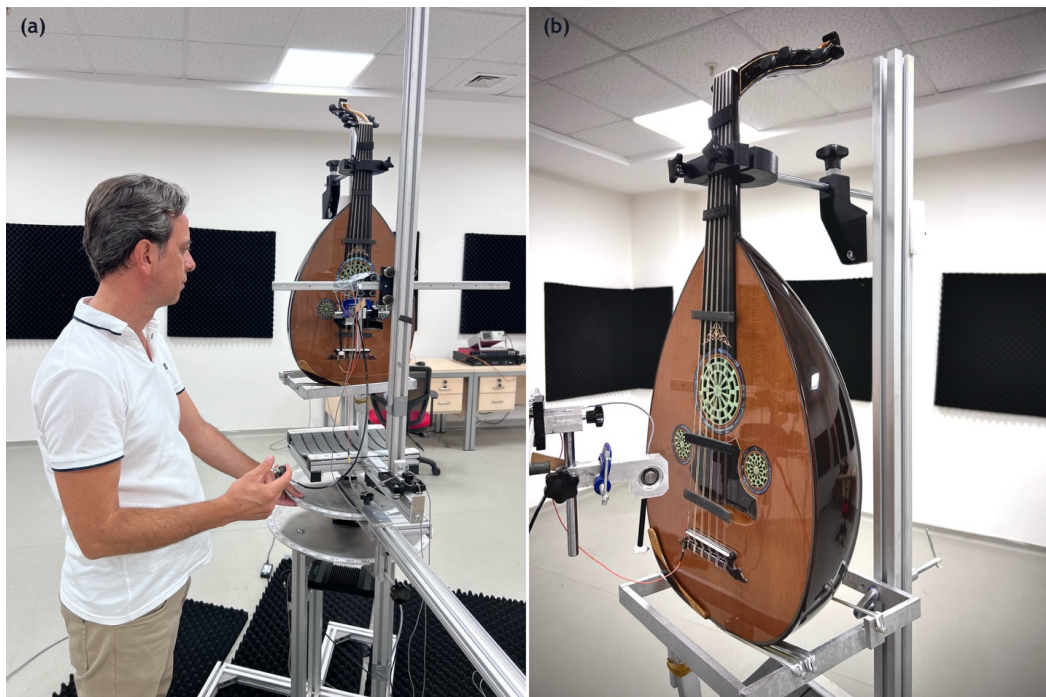
Photo 1. Experimental oud and measurement setup: (a) impact-hammer excitation applied to the bridge via an extension arm; (b) oud mounted in the experimental fixture (Author's personal archive).
