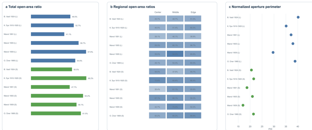
Figure S3. Comparison of total openness, regional openness, and normalized aperture perimeter P/D for the traditional reference geometries. P/D is provided only as a dimensionless geometric descriptor
