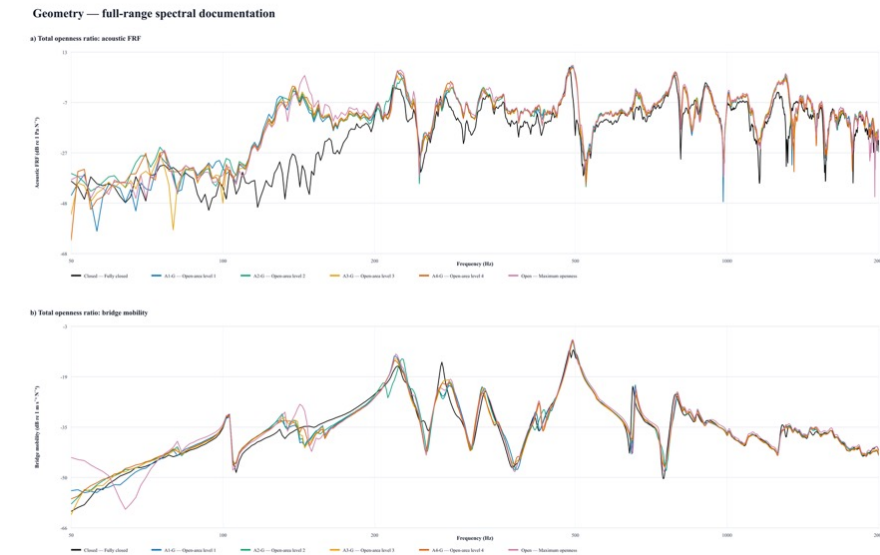
Figure S9. Full-range force-normalized acoustic FRF and bridge-mobility spectra for the total open-area ratio series, ordered from Closed through A1-G-A4-G to Open (50-2000 Hz; logarithmic frequency axis)
