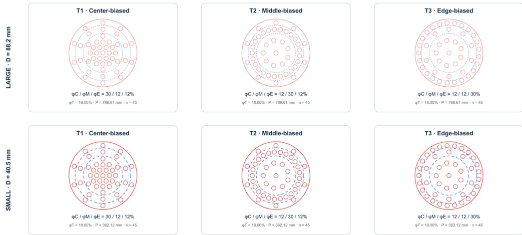
Figure S5. Regional open-area distribution series. The total open area, total aperture-edge length, aperture count, and aperture diameter are controlled within a diameter; only the radial location of the high-open-area zone is changed.
