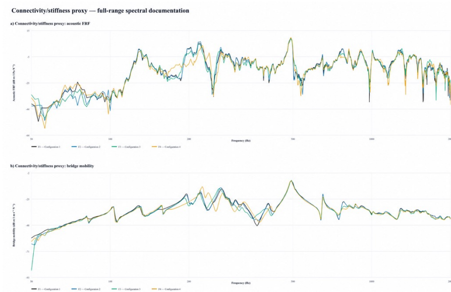
Figure S13. Full-range force-normalized acoustic FRF and bridge-mobility spectra for the connectivity/stiffness-proxy configurations F1-F4 (50-2000 Hz; logarithmic frequency axis)
