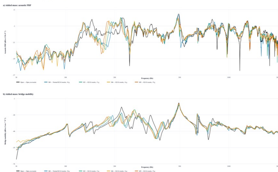
Figure S12. Full-range force-normalized acoustic FRF and bridge-mobility spectra for the physical added-mass sequence Open, M0, M3, M6, and M9 (50-2000 Hz; logarithmic frequency axis)
