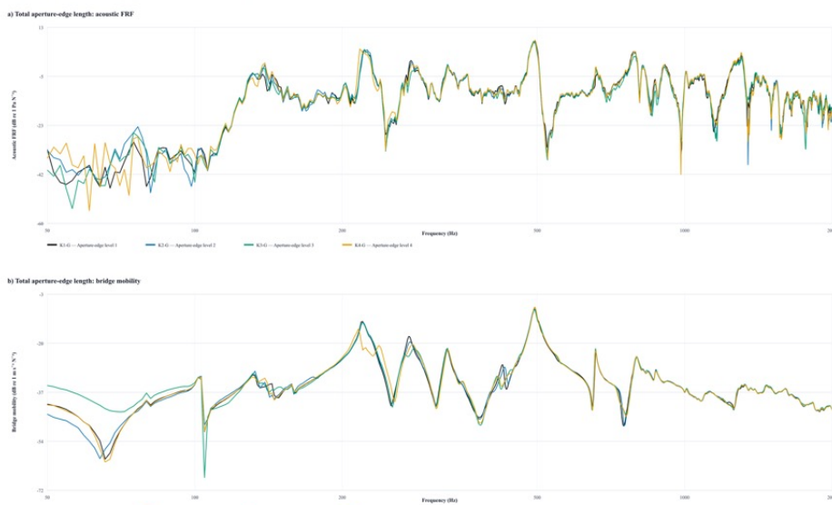
Figure S11. Full-range force-normalized acoustic FRF and bridge-mobility spectra for the total aperture-edge-length series K1-G-K4-G (50-2000 Hz; logarithmic frequency axis)
